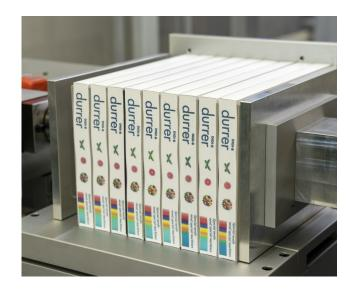
The DIGI-B is a digital colour cutting machine for industrial production. The printing of 4 sides is possible in a fully automatic process. The pre-stacking of the products takes place during the printing process on a separate device. The complete stack is loaded in insert/delivery station in the clamping device.
