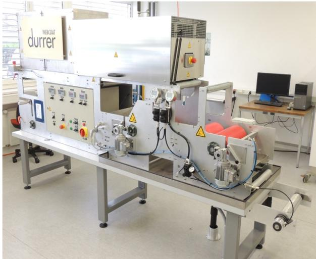
The D300 Web Coater corresponds with the latest technological standards in the industry. The machine enables the coating process to be reproduced very realistically in the laboratory. The comprehensive setting options allow individual formulations to be tested and optimised. The knowledge gained can then be applied on the production machine with high process capability.
