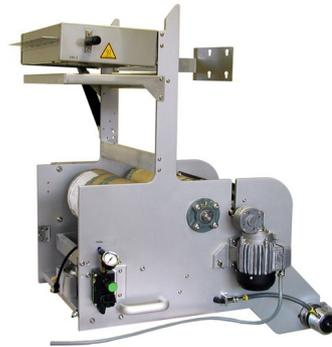
The paper is fed through a gap between the rollers, thereby applying the coating colour to the paper. The coating colour has previously been applied to the roller as a "film" by means of the roll squeegee. This film is then transferred from the roller on to the paper as it passes through the gap.
